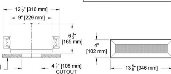
NOTE: This option is intended for use with precise and finished cutouts. There is no plaster or finish flange.
