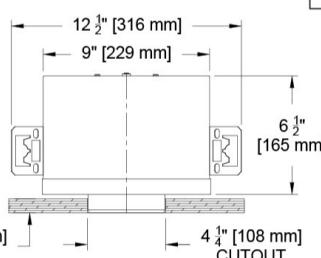
NOTE: This option is intended for use with precise and finished cutouts. There is no plaster or finish flange.
