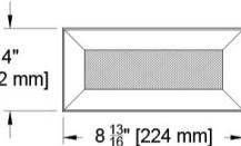
NOTE: This option is intended for use with precise and finished cutouts - usually millwork or wood ceilings. There is no plaster or finish flange.
