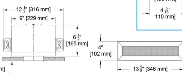
NOTE: This option is intended for use with precise and finished cutouts - usually millwork or wood ceilings. There is no plaster or finish flange.
